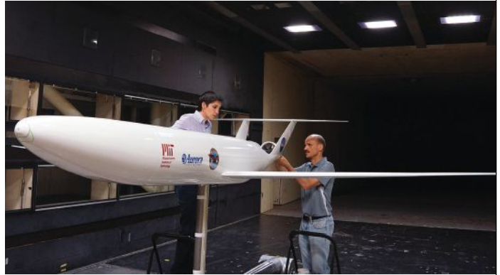
MIT and NASA engineers test a 1/11th scale model version of the D8 airliner concept in the 14-by-22-ft. Subsonic Wind Tunnel at NASA's Langley Research Center. Image courtesy of NASA Langley/Kathy Barnstorff.
