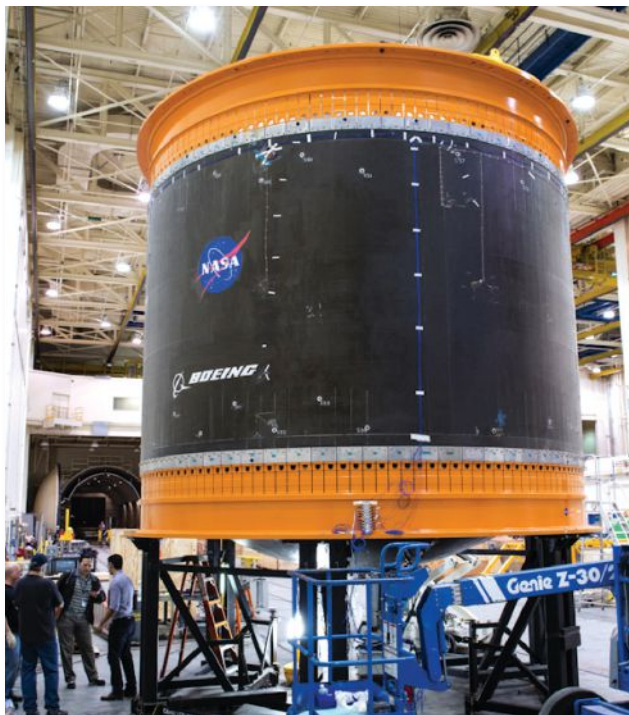
One of the largest composite rocket propellant tanks ever manufactured is prepared for transport on NASA's Super Guppy airplane. Image courtesy of The Boeing Co.
